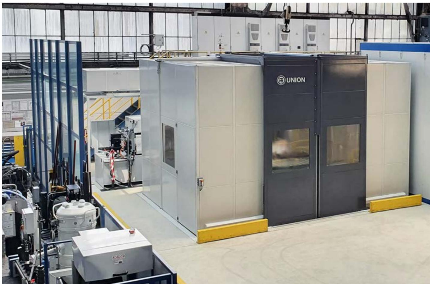
The T-Series CNC horizontal boring and milling machine for effective and economical machining of medium-heavy workpieces (up to 10 t) with a working area of up to 2,500 × 2,000 × 1,600 mm
