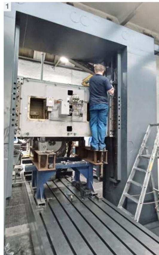
1. Important components and wear parts of the portal milling machine have been conscientiously checked and overhauled by our experts
