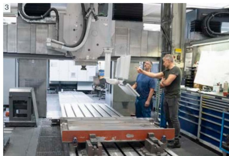
2. The outdated machine control system (at the top front of the picture), just like the software, is being brought up to date
