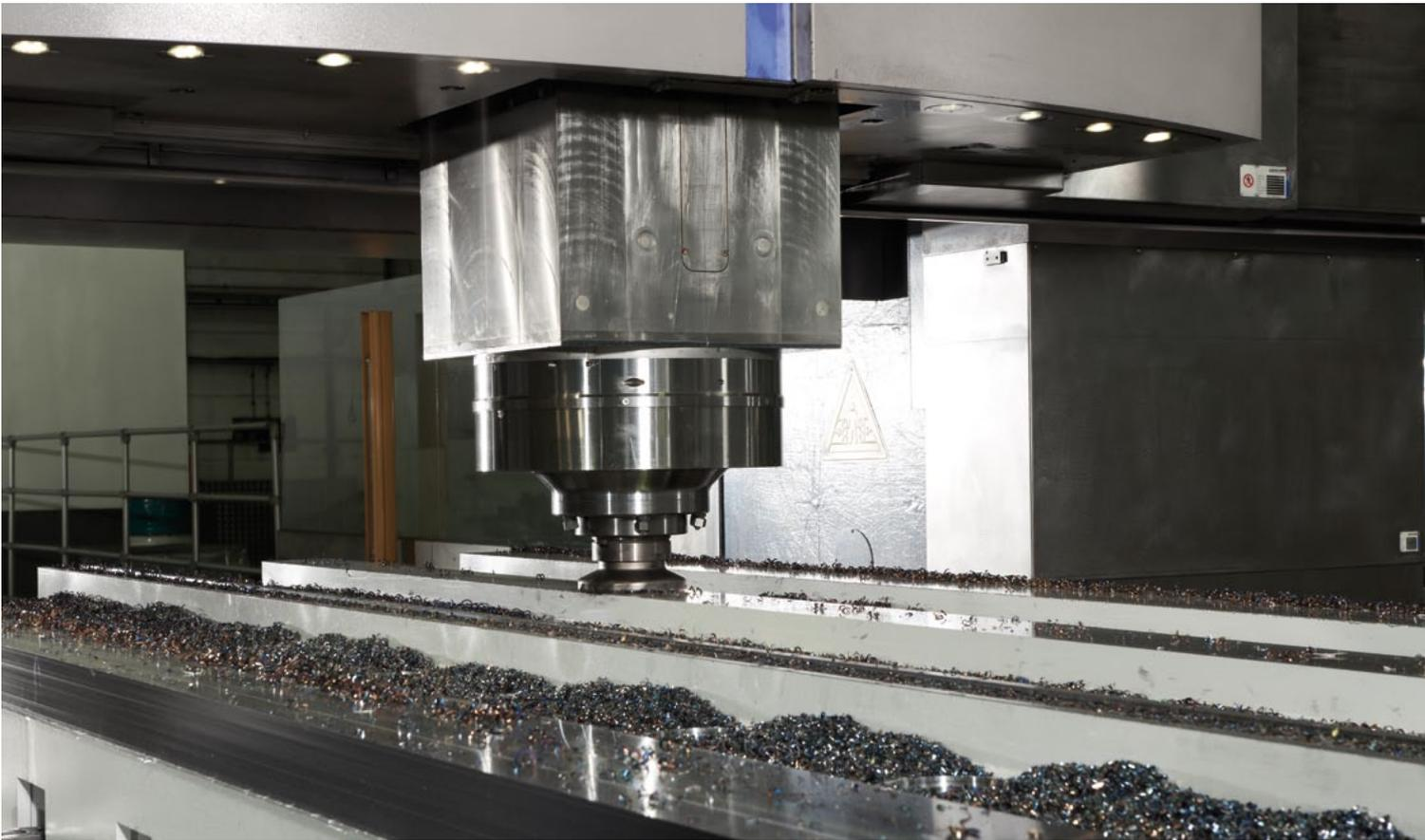
Machining a machine bed
