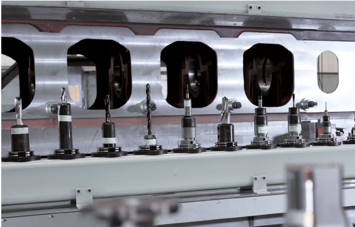
Automatic tool changing system with 192-pocket racks
