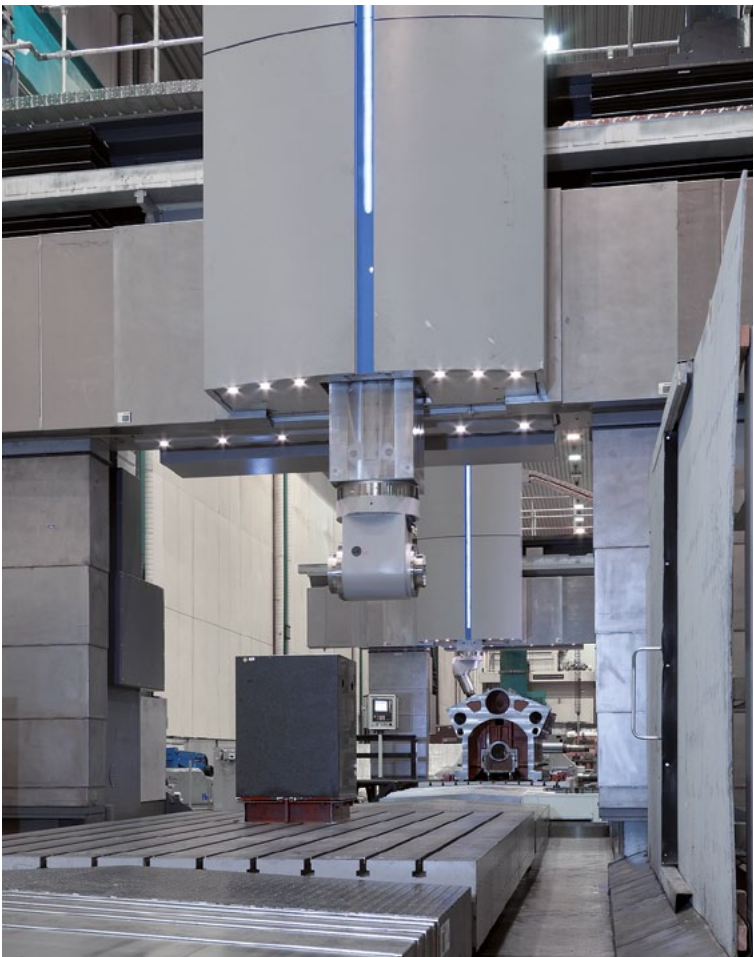
Two ProfiMill portal milling machines with a milling power of 100 kW at the tool center point
