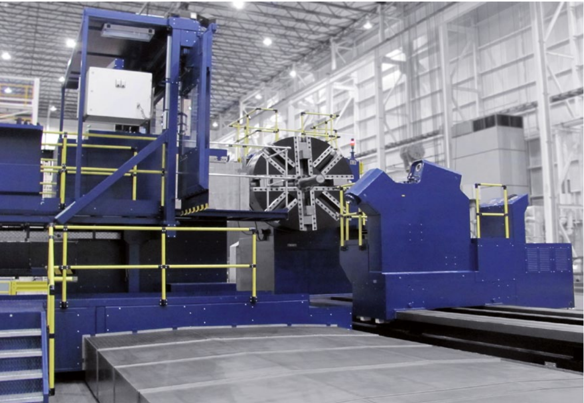
The ProfiTurn H operates with an axial and radial runout tolerance of 5 µm
