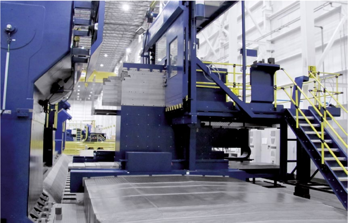
The carriage is driven by a preloaded double pinion drive
