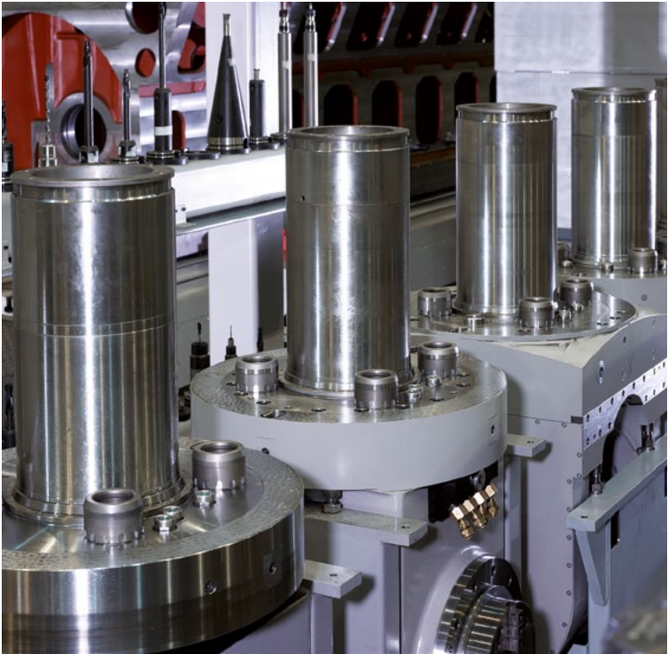
The portal mills are equipped with eight special milling units each
