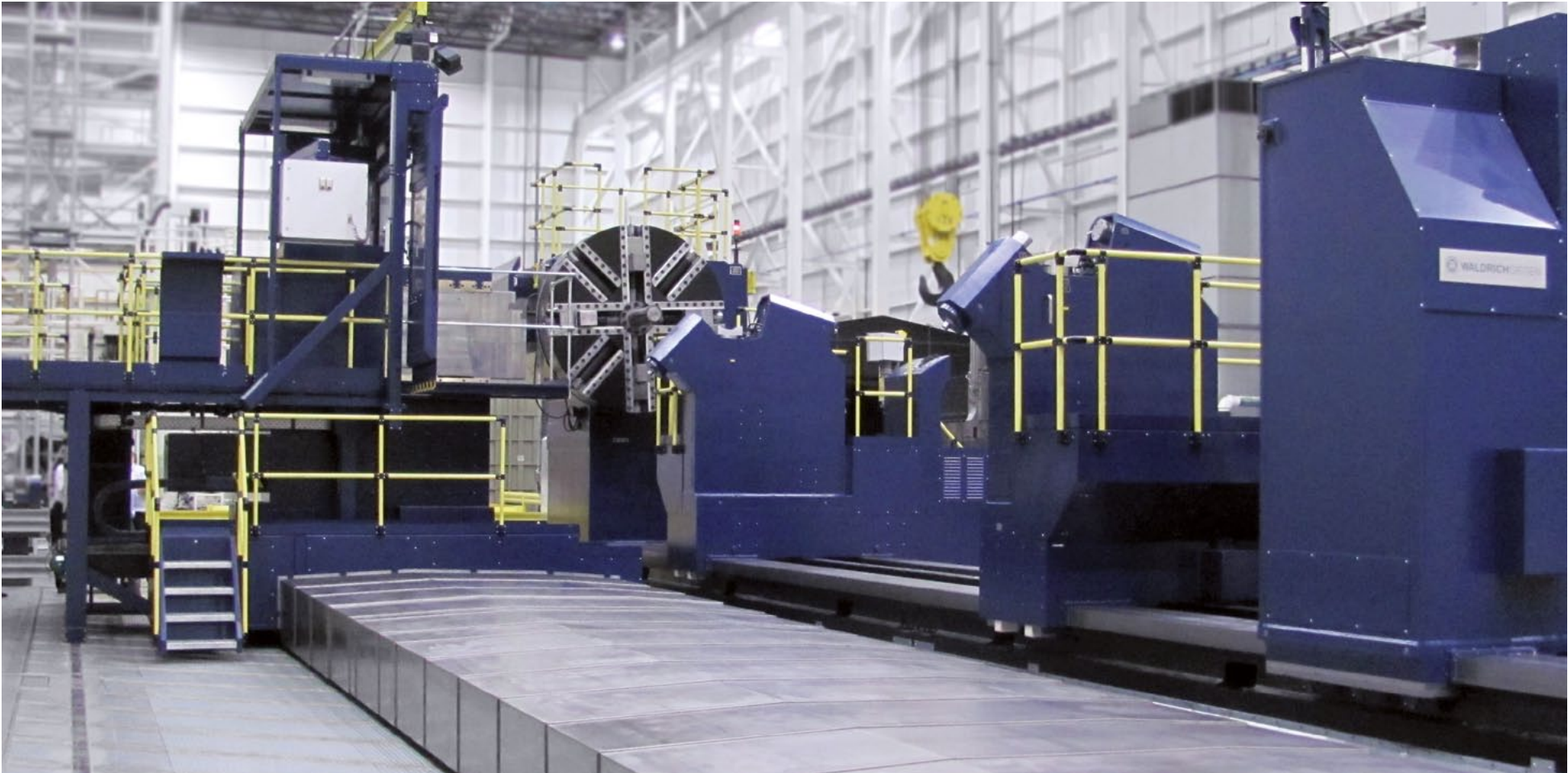
ProfiTurn H with a drive power of 310 kW and a torque of 200,000 Nm
