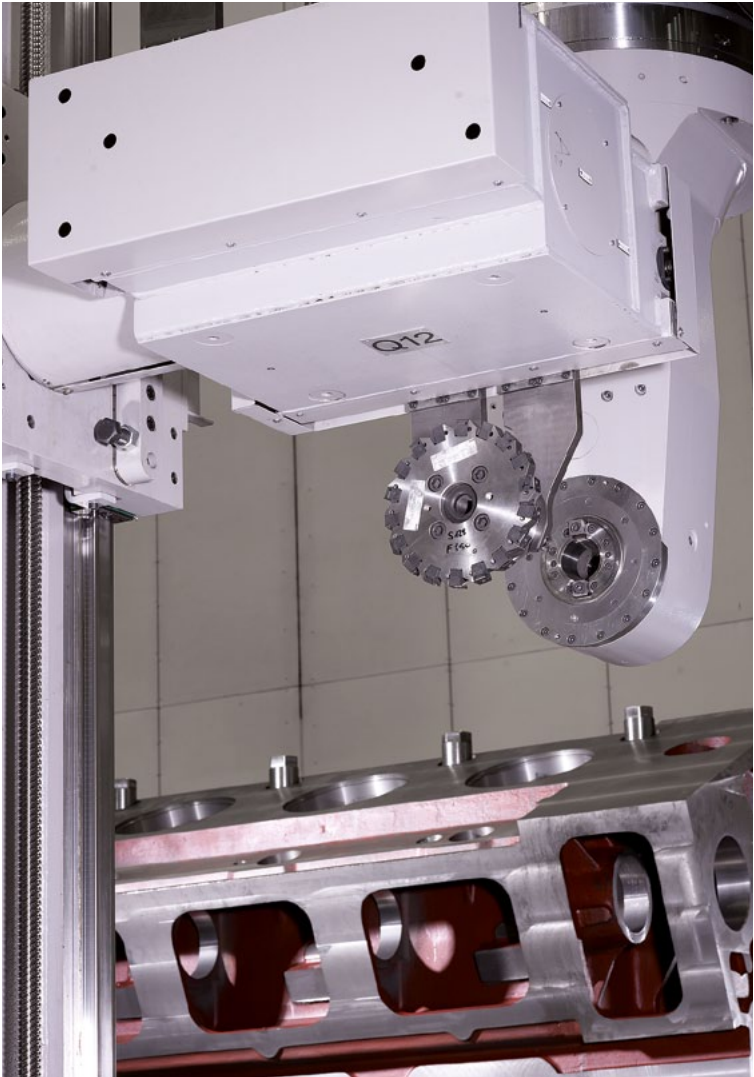
Switching between machining applications with an automatic tool changer
