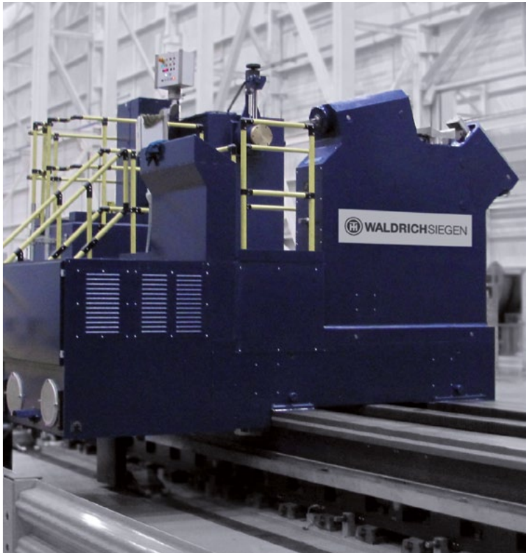
The rotors are turned in hydrostatic steady rests
