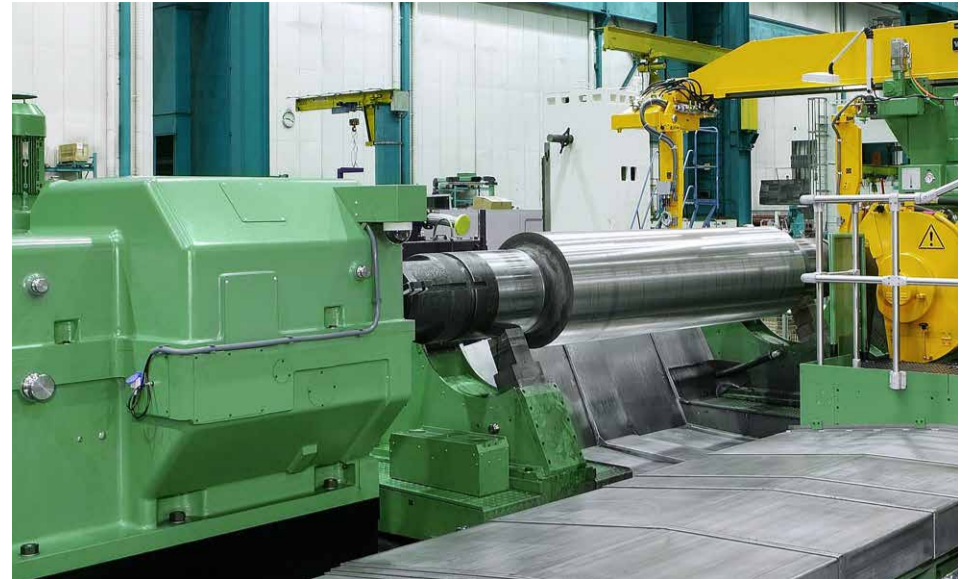
As good as new: roll grinder after complete modernization
