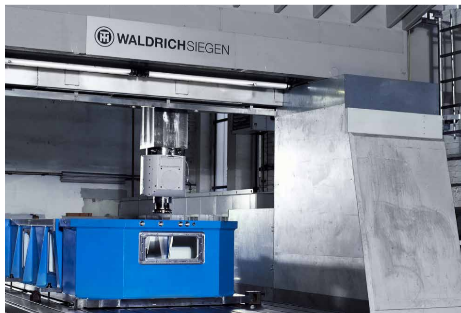
The optional concrete column further enhances the machine's stiffness
