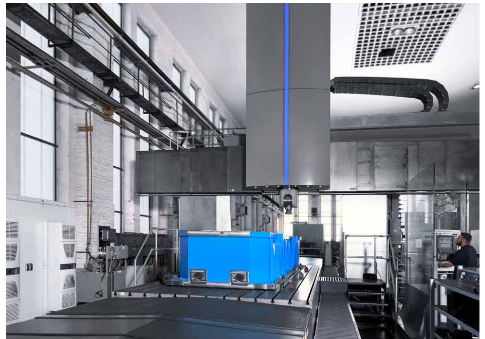
The ProfiMill 1 machines the housing of an XXL helicopter test bench gearbox
