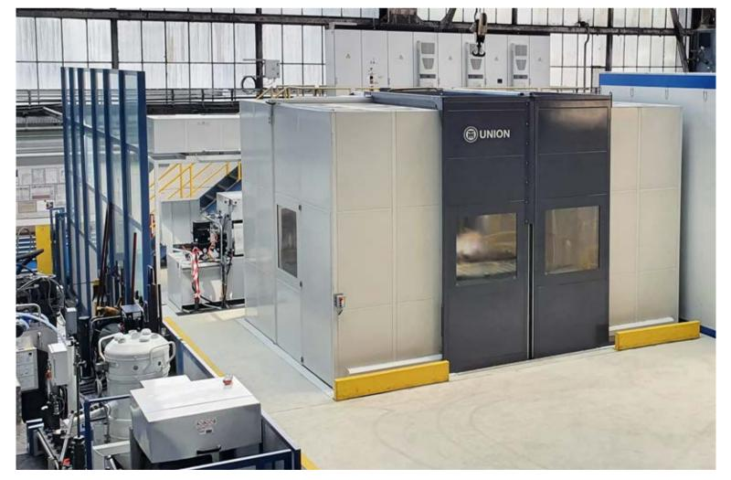
The T-Series CNC horizontal boring and milling machine for effective and economical machining of medium-heavy workpieces (up to 10 t) with a working area of up to  $2,500 \times 2,000 \times 1,600$  mm
