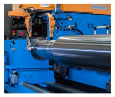
ally machine back-up and intermediate rolls with and without chocks with a roll length of up to 7,000 mm and a maximum weight of 55 t," says Jannik Schneider. Another special feature is that, in addition to conventional grinding, smaller turning operations can also be carried out on new rolls thanks to the turning tool holder.
